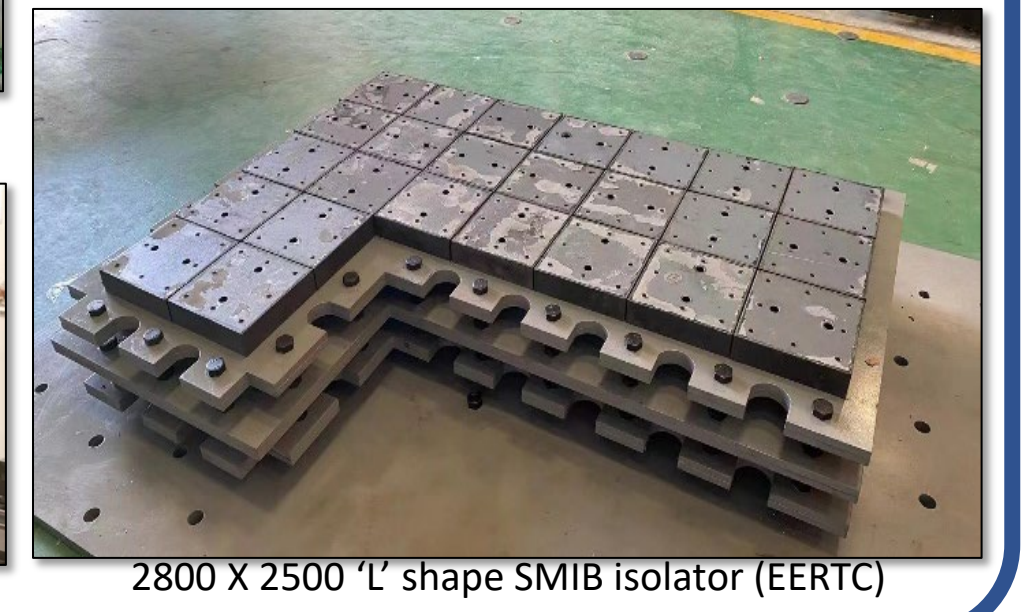
2800 X 2500 'L' shape SMIB isolator (EERTC)
