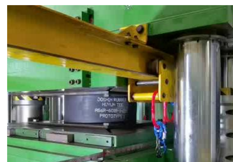
Dynamic reduced-scale test example (AS6R)
