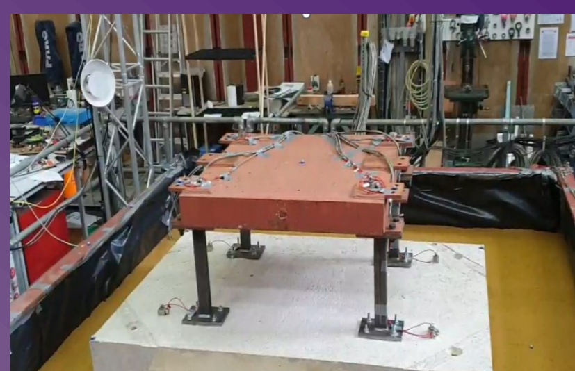
Large-scale shaking table tests
